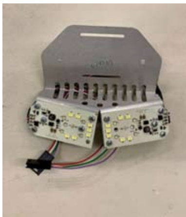
Figure 3 - Slush machine disinfection system. The nUV light sources (yellow LEDs) were mounted on an angled PCB holder to uniformly irradiate the inner and front sections of the tank. Light uniformity was also optimised by positioning the LEDs on the PCB.
