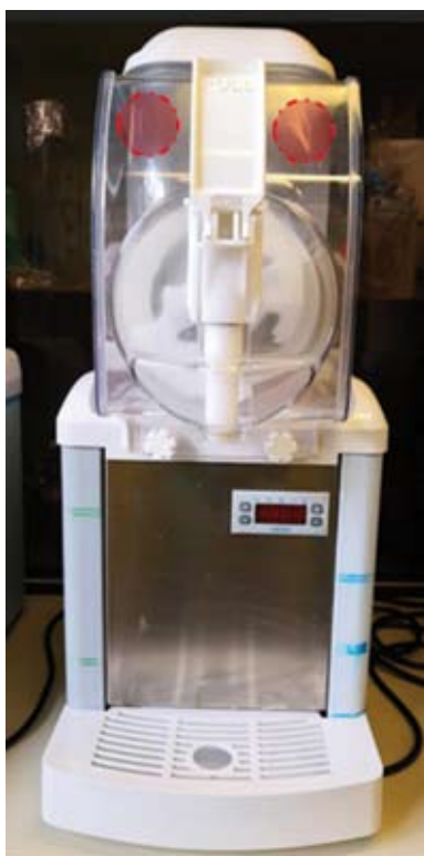
Figure 1 - SP1 Slush machine front view. In red, the inner front sections of the tank spread with contaminated slush.
