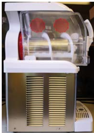
Figure 2 - SP1 Slush machine lateral view. In red, the inner lateral sections of the tank spread with contaminated slush. The inner section of the tank was contaminated using a special stamp to facilitate the adhesion of the contaminated slush to the walls.
